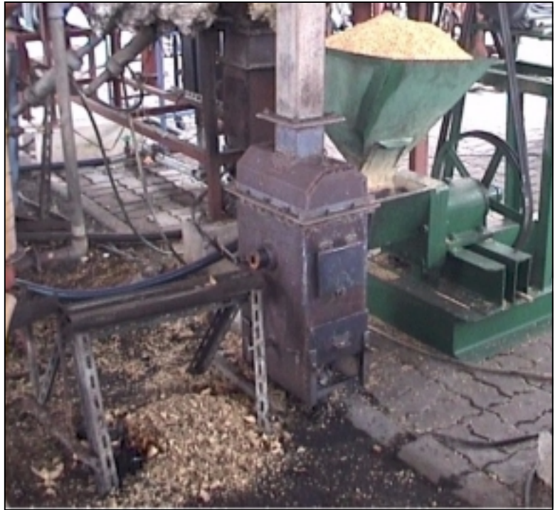
Figure 4: Biomass die-heating stove in operation
